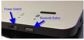
\*Note the Power is on the left and is a <u>Switch</u> that moves right and left, whereby the Bluetooth is a <u>Button</u> that can only be pushed in. **DO NOT TRY AND MOVE THE BUTTON UP/DOWN/FORWARD/BACK.**
